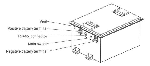
Note: Press and hold the "MAIN SWITCH" button for 3 seconds to turn on/off the battery, green light indicates power on.
